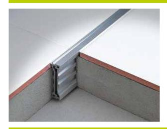
COFLEX CKM technical sliding expansion joints are conceived for thin-set installations. Two metal sides interlock and slide with an internal gap of +/-3/32" (2mm), redistributing differential movement due to material compression and expansion. The profile comes assembled in a "neutral" position, held together by an elastic gasket in the lower profile section. It offers durability and high resistance to vertical loads with a modern design. Suggested floor bays: 172-7/32" -269-3/32"ft² (16-25m²).
